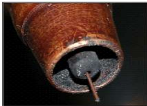
Figure 1 Spatters on the contact tip.
